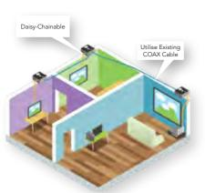
Homes want HDMI but are stuck with coax. The solution? The DIGI-HD-COAX distributes 1080p HDMI over a single RG59 or RG6—just plug it into the wall and go! Plus, built-in amplified splitters provide seamless integration between rooms.
